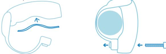
**CAUTION** Regularly check that your sensor is well positioned and always adjusted to the fork.
